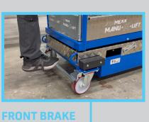
Single bar brake needed to lock the wheels before use
